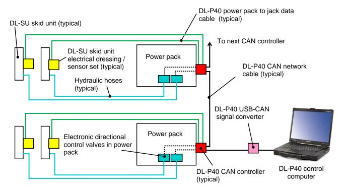
The main features of the DL-P40 computer control system are as follows:
