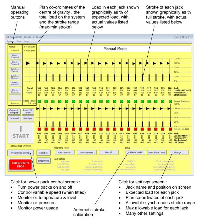
The operator can select any combination of jacks to operate and presses the Sychro Extend and Sychro Retract buttons to lift and lower the load. The system will automatically synchronise all the jack stokes to maintain the required level of stroke synchronisation. A log file of all jack loads, user commands and warnings is automatically saved for every operation and the operator can comment to the log file at any time using the 'comment to log file' button.
